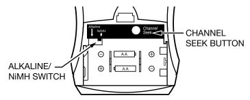
5. To lock or unlock a selected channel, turn the power off. While holding the seek button, turn the power back on. When locked, the receiver will remain on the current channel, regardless of channel seek button presses.
