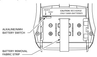
Install the AA batteries. Be sure to observe proper polarity (+/-). Damage due to improper battery installation may void the warranty on the product.
