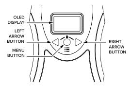
4. Change the receiver to the channel/frequency chosen in step 3. Push the menu button once and select the channel by pushing the left or right arrow buttons. (Figure 7).
